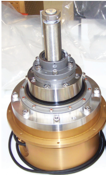
Figure 1: Actuation for hexapod struts including harmonic drive / servomotor (partially concealed within gold alodine housing) and recirculating roller screw
