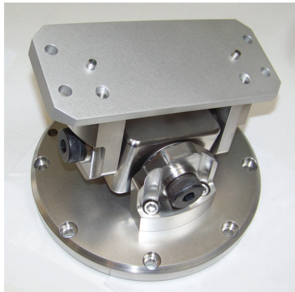
Figure 2: Custom 2-DOF universal joint uses tapered roller bearings and closely approximates an ideal end-joint for telescope positioning applications
